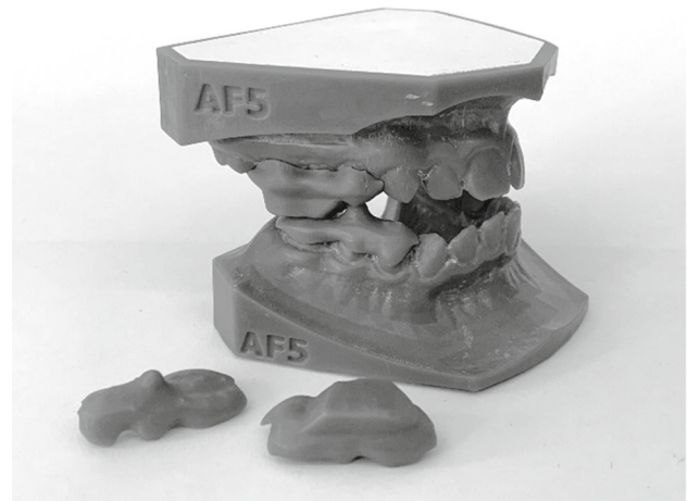
Fig. 6 The additively manufactured prototype of the device
