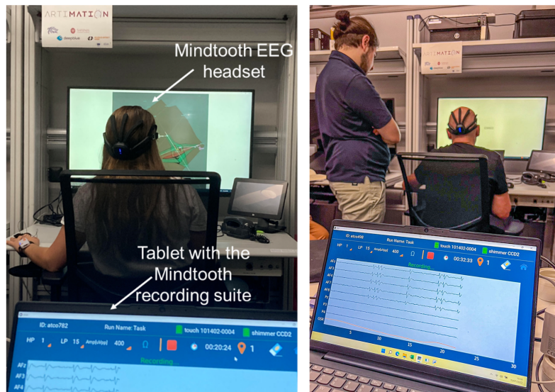
Fig. 4 Validation setup for the neurophysiological measures.
